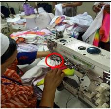
Rotating belt without protection. The worker could touch the belt and be seriously injured. The factory should cover any moving element of the machines.
