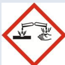
GHS05 Danger or Warning / Corrosive cat. 1
