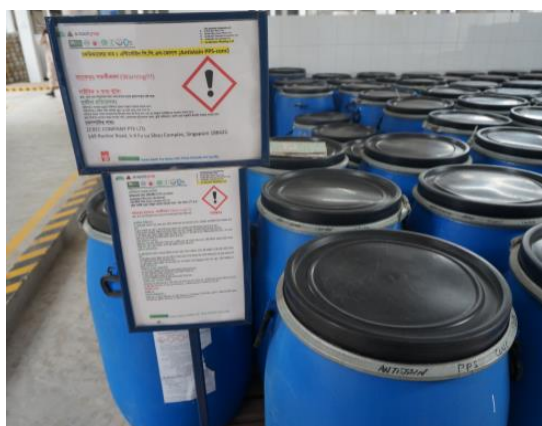
Pictures 1 and 2: examples of SDS in local language available nearby the chemical containers. Picture 1: in a chemical warehouse. Picture 2: in the storage area for chemicals used for the Effluent Treatment Plant (ETP). Wherever chemicals are used, SDS must be available and easily accessible.
