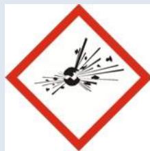
GHS01 Danger / Unstable, Explosive
