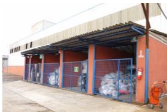
Picture 1: dedicated shed for hazardous waste with different sections for different waste types. The storage area is covered to prevent rainwater ingress. The access to each section is restricted.
